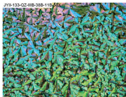
Figure 3. Polarized optical micrograph of 7 cooled to room temperature from the mesophase (250 \mu\text{m} \times 190 \mu\text{m} ).
